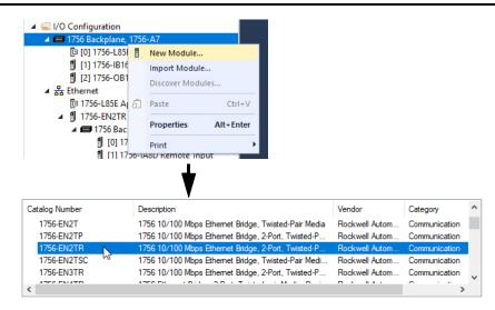
8. Since the I/O now has to reside in a separate chassis, add another EtherNet/IO adapter under the adapter you just created.
