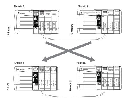
The difference between a locked switchover and a normal switchover is that you initiate the locked switchover. You or a fault in the primary chassis initiate a normal switchover.
