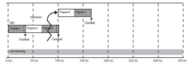
Figure 12 - Watchdog Configured for Redundancy Switchover
