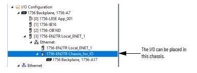
9. Copy the I/O modules and paste them into the chassis of the newly added communication module.
