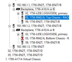
To correct the missing module anomaly, first verify that the redundancy module is correctly installed in the chassis and it is properly powered. Then check the intermodule cable that connects the redundancy modules.
