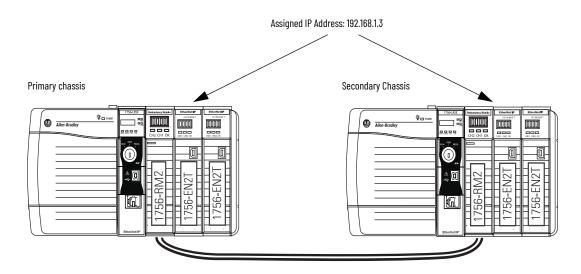
When a redundancy system begins operating, the primary EtherNet/IP communication module uses the IP address that is assigned during initial configuration. The secondary EtherNet/IP communication module automatically changes its IP address to the next highest value. When a switchover occurs, the EtherNet/IP communication modules swap IP addresses.
