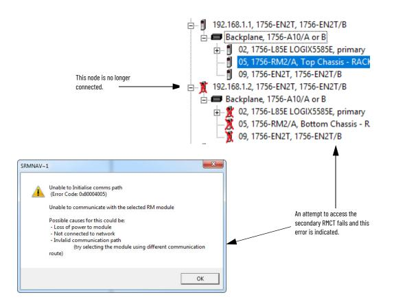
To recover from a EtherNet/IP<sup>™</sup> network disconnection, perform the following:
