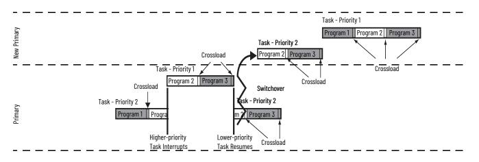
The following diagram shows a lower priority task that has not been completed and a switchover occurs. The lower priority task and programs are executed from the beginning and not at the program where the switchover occurred. This result is because the crossloads and synchronization points were not configured to occur at the end of each program.
