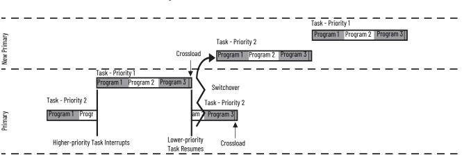
Figure 10 - Periodic Task Execution After Switchover When Configured Not to Crossload After Programs
