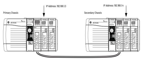
Figure 3 - IP Addresses of EtherNet/IP Communication Modules After System Operation Begins
