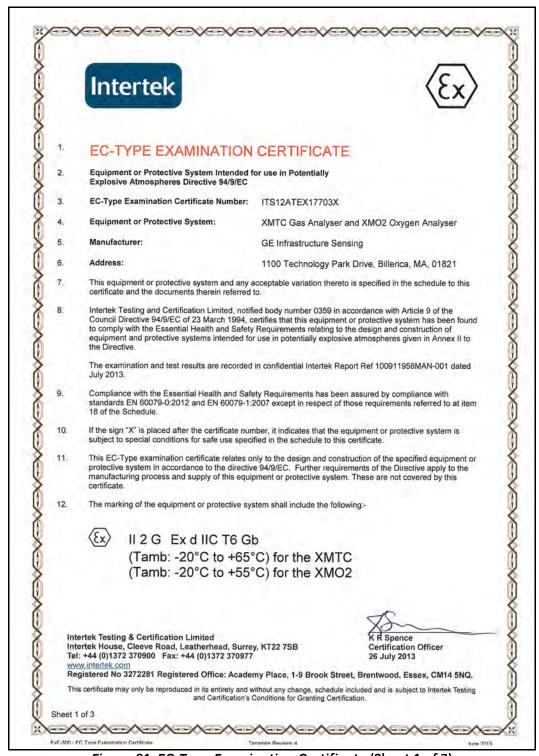
Figure 91: EC-Type Examination Certificate (Sheet 1 of 3)
