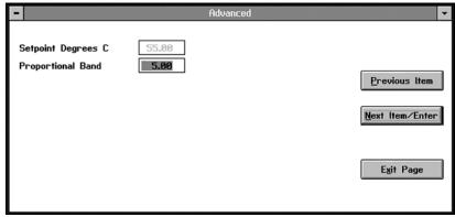
Figure 76: Proportional Band in the Heater Window
