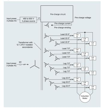
Figure 2.8 Pre-charge component connection diagram.
