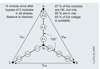
Figure 2.6 Drive output rebalanced by bypassing functional cells
