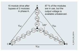
Figure 2.5 Drive output with 2 cells bypassed in phase A
