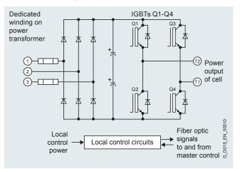
Figure 2.3 Schematic of a typical power cell.
