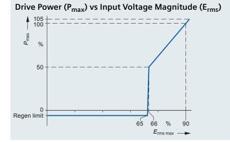
Figure 5.1 Drive power ( $\rm P_{max})$  as a function of input voltage magnitude ( $\rm E_{rms})$
