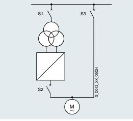
Figure 4-1 Circuit-breakers/contactors
