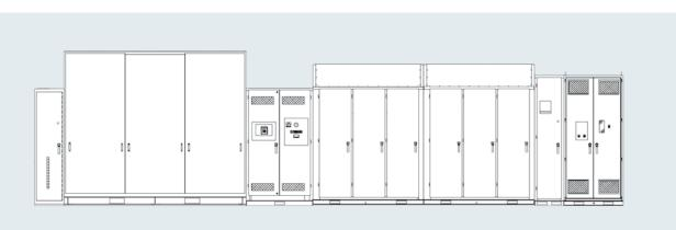
WCIII for motor voltages 3.3 to 7.2kV; schematic drawing A
