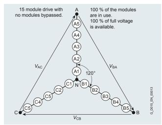
Figure 2.4 Simplified diagram of a 15 cell drive
