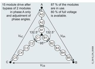
Figure 2.7 Drive output rebalanced by adjusting phase angles (Neutral Shift).
