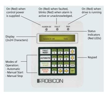
Figure 5.2 The operator panel of the ROBICON Perfect Harmony drive series
