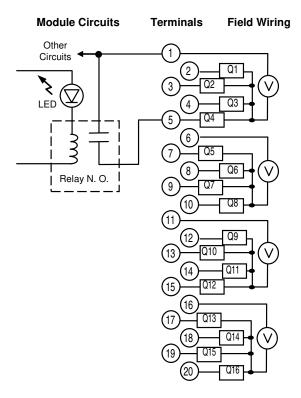
Screw terminals accept two copper wires in the range AWG #22 (0.36 mm²) to AWG #16 (1.3 mm²), or one AWG #14 (2.1 mm²) copper 90°C (194°F) wire. Each terminal can accept solid or stranded wires, but the wires into any given terminal must be the same type (both solid or both stranded) and the same size. Screw torque is from 9.6 in-lbs to 11.5 in-lbs (1.1 to1.3 Newton-meters).
