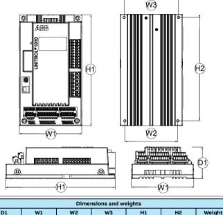
W1 W3 H1 H2 Weight D1 mm in mm in mm in mm in kg lb mm in mm in 85 3.3 170 6.7 143.5 5.6 147.5 5.8 302 11.9 280 11.0 2.8 6.2
