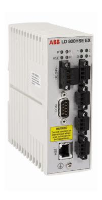
The FOUNDATION Fieldbus Linking Device LD 800HSE EX is registered according to class 42c of the HSE profile, therefore providing the following functions:
