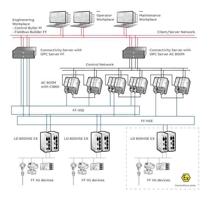
Figure 1. Sample System Structure with FF Network
