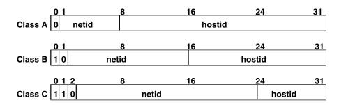
In general, the *netid* part is assigned by the Internet authorities and the *hostid* part is assigned by your local network administrator. The class of network determines the number of hosts that can be supported. A Class A network can support  $2^{24}$ -2 (16,777,214) hosts, Class B,  $2^{16}$ -2 (65,534) hosts, and Class C,  $2^{8}$ -2 (254) hosts. The minus 2 refers to host numbers reserved for the network itself and the local broadcast.
