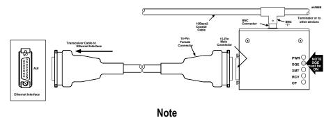
Transceivers must be compatible with the IEEE 802.3 standard and must have the SQE option Enabled.
