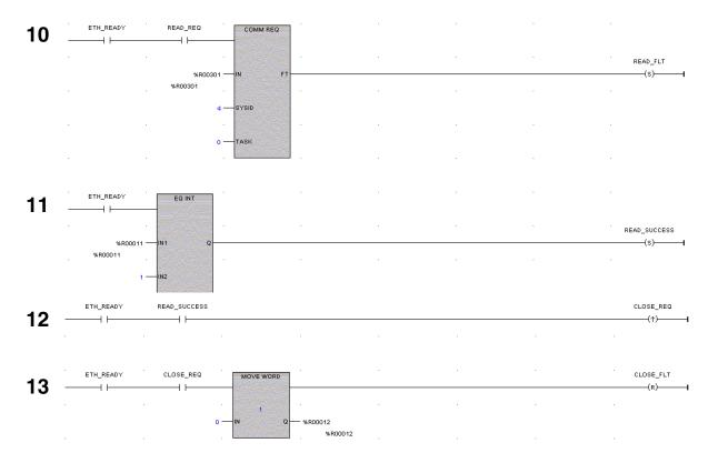
**Rung # 10**: The COMMREQ Function Block has three input parameters and one output parameter.
