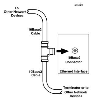
Connecting the CMM742 Ethernet Interface to a 10Base2 Network with "F" Connector
