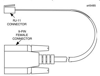
If your terminal or PC is unable to communicate with the Ethernet Interface through the RS-232 port, consult the documentation for your terminal or PC to verify that your connection is wired correctly.
