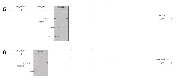
**Rung # 5**: The COMMREQ Function Block has three input parameters and one output parameter.
