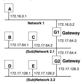
Here, a second network with Hosts D and E has been added. Gateway G2 connects Subnet 2.1 with Subnet 2.2. Hosts D and E will use Gateway G2 to communicate with hosts not on Network 2.2.
