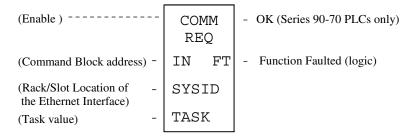
Each of the inputs and outputs are discussed in detail below. Remember that the Command Block address points to a location in memory that has been set up as the Command Block.
