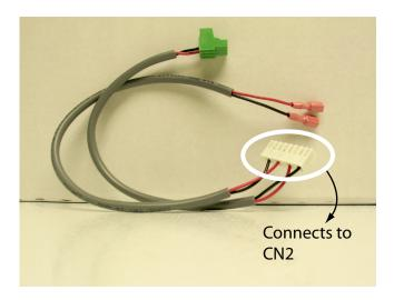
Figure 3: 12VDC Power and Battery Cable Assembly
