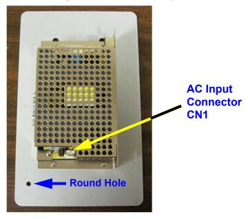
7. Slide the power supply down in the keyholes until they bottom out. Then, tighten the four mounting screws to secure the power supply to the metal plate.
