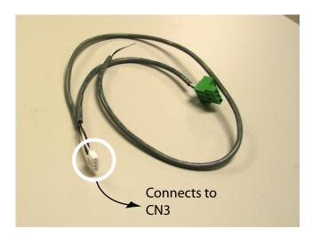
Figure 4: AC and Battery Fail Cable Assembly
