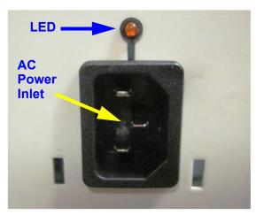
11. Connect the AC power inlet and LED indicator cable to the power supply by pushing and inserting the cable connector to the pin connector **CN1**:
