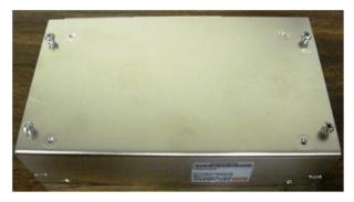
6. Position the power supply over the 4 keyholes on the metal plate making sure that the round hole (see the below figure) is in the bottom left corner as shown and the power supply is positioned with the AC input terminals (CN1) facing downward.
