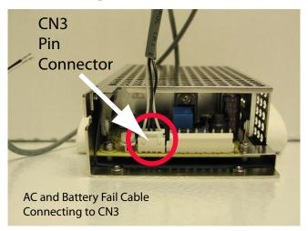
This is how the pin connectors CN2 and CN3 should look like after attaching both cables:
