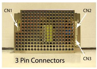
Figure 1: Power Supply Pin Connectors
