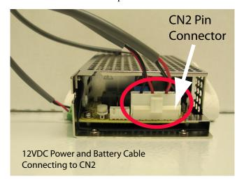
Figure 7: 12VDC Power and Battery Cable Assembly Connecting to CN2 Pin Connector
