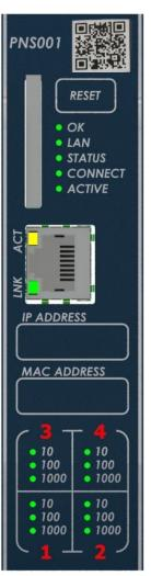
**Note:** Under certain ambient operating temperatures, the PROFINET Scanner could momentarily display the over temperature pattern during power up, while it is calibrating its thermal protection functions. This indication can be ignored. For details, refer to the section entitled *Microprocessor Over-Temperature* in *PACSystems RX3i PROFINET Scanner Manual*, GFK-2737.
