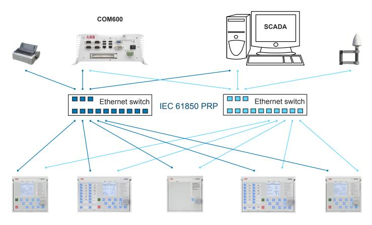
Figure 22. Parallel redundancy protocol (PRP) solution
