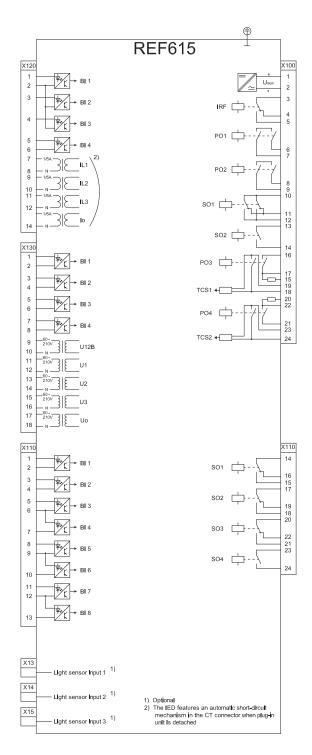
Figure 34. Terminal diagram of standard configurations H, J and N
