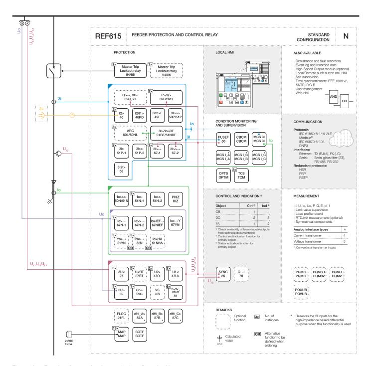
Figure 12. Functionality overview for standard configuration N
