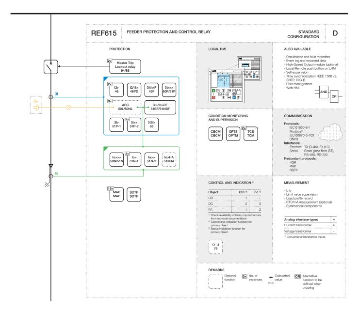
Figure 4. Functionality overview for standard configuration D
