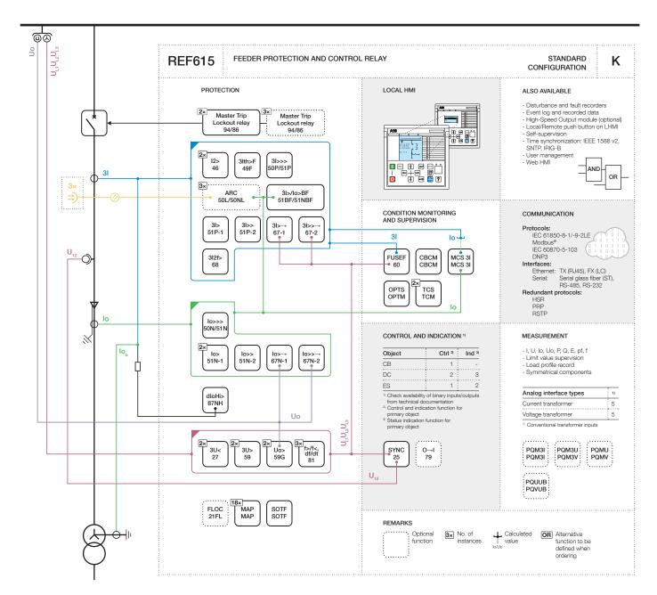
Figure 10. Functionality overview for standard configuration K
