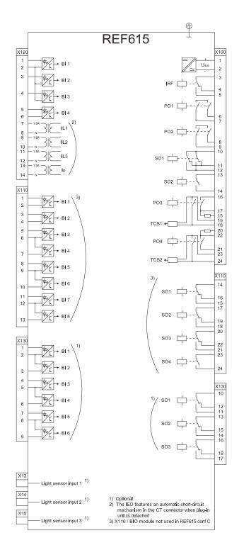
Figure 31. Terminal diagram of standard configurations C and D
