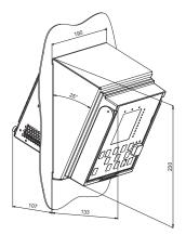
Figure 29. Semi-flush mounting in a 25° tilt
