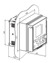
Figure 28. Semi-flush mounting
