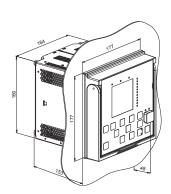
Figure 27. Flush mounting
