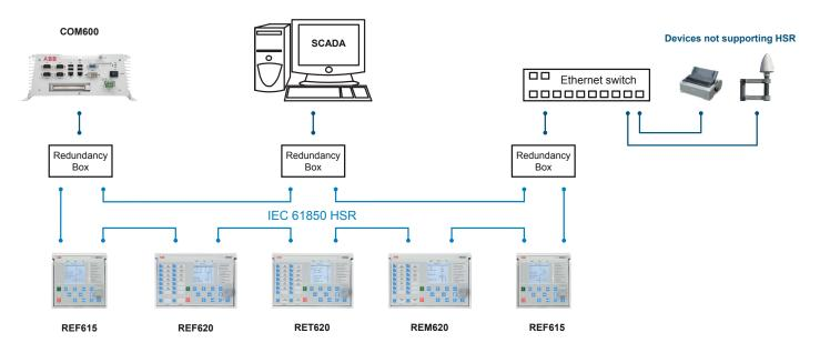
Figure 23. High availability seamless redundancy (HSR) solution
