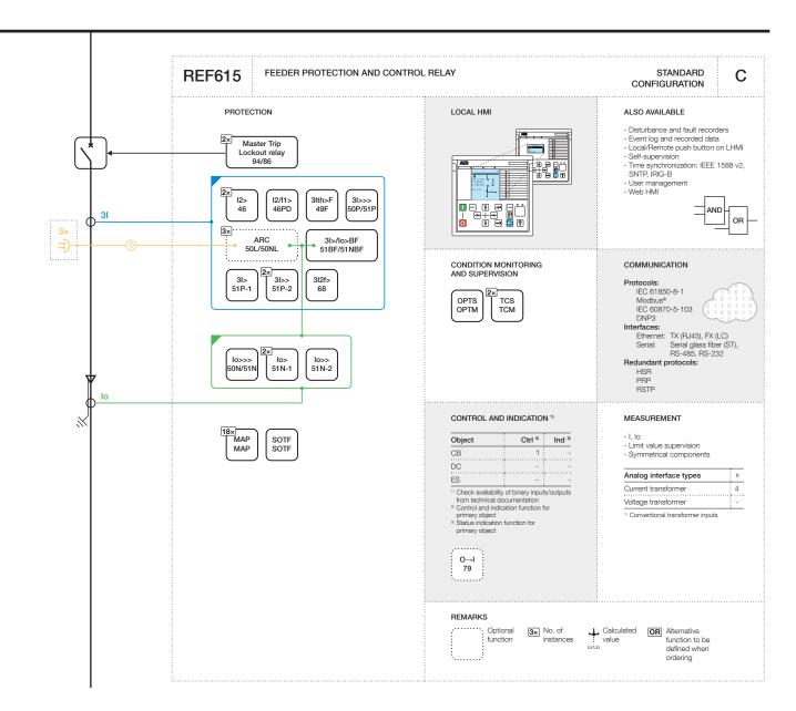
Figure 3. Functionality overview for standard configuration C
