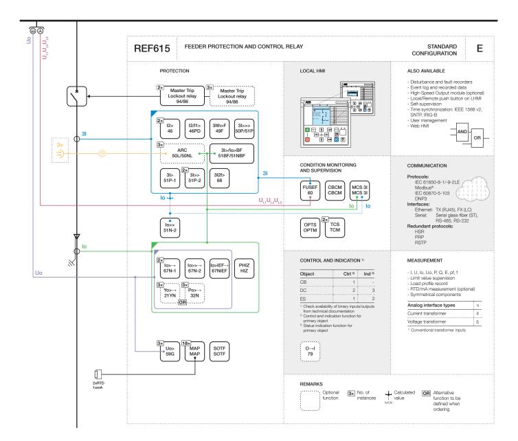
Figure 5. Functionality overview for standard configuration E
