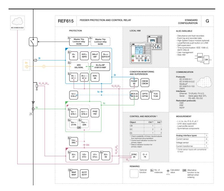
Figure 7. Functionality overview for standard configuration G
