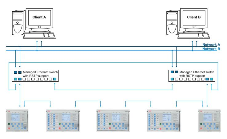
Figure 24. Self-healing Ethernet ring solution
