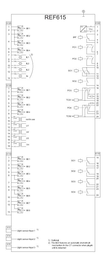
Figure 32. Terminal diagram of standard configurations E and F
