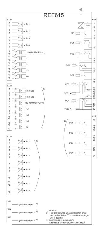
Figure 35. Terminal diagram of standard configuration K
