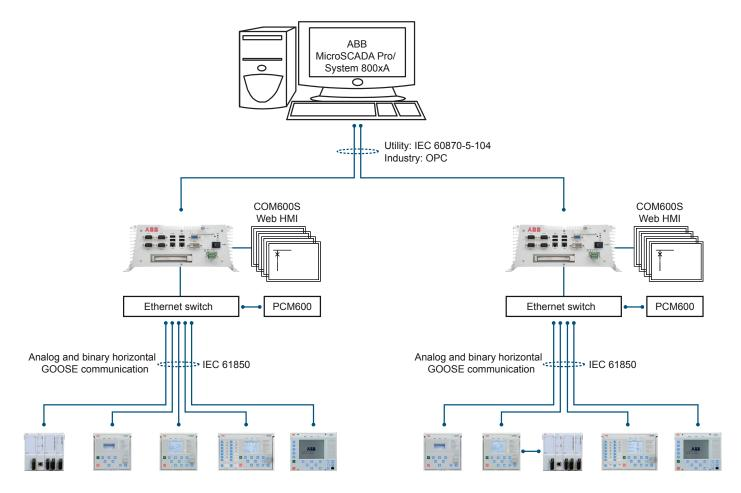
Figure 20. ABB power system example using Relion relays, COM600S and MicroSCADA Pro/System 800xA
