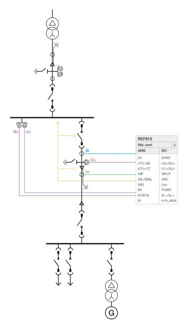
Figure 18. Protection and control of outgoing feeder with standard configuration J
