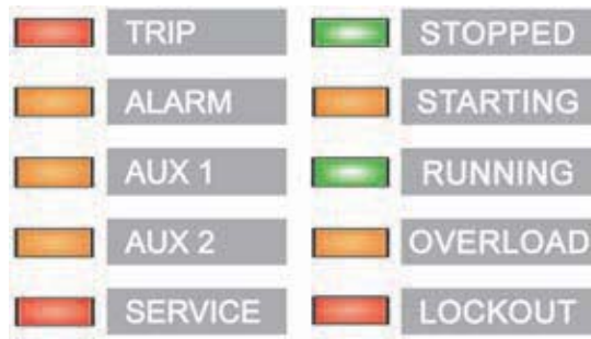
FIGURE 4-1: LED Indicators - Enhanced Faceplate
