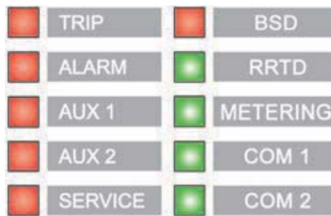
FIGURE 4-2: LED Indicators - Basic Faceplate
