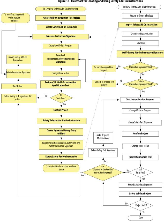
Figure 18 - Flowchart for Creating and Using Safety Add-On Instructions
