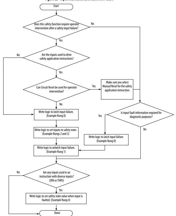
Figure 22 - Input Fault Latch and Reset Flow Chart
