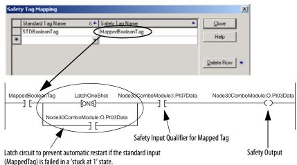
Figure 14 - Qualify Standard Data with Safety Data
