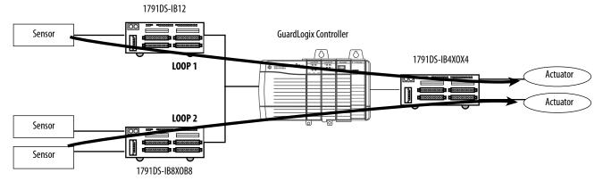
To determine the logic element PFH for each safety loop in the simple example system shown in the PFH Example, sum the PFH values for each component in the loop. The PFH Equations by Safety Loop table provides a simplified example of PFH value calculations for each safety loop shown in the PFH Example illustration.
