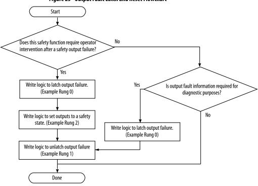
Figure 25 - Output Fault Latch and Reset Flowchart
