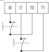
For Cat 1, Cat 2, and SIL 2 safety functions, the Guard I/O safety modules need specific configurations within the GuardLogix project. In this example, inputs 0, 1, 6, 7, 8, 9, 10, and 11 are part of a CAT 1, 2 or SIL 2 safety function, because they are configured as Single. Inputs 2 and 3, as well as 4 and 5 are part of a CAT 3, CAT 4, or SIL 3 safety function, because they are configured as Equivalent.
