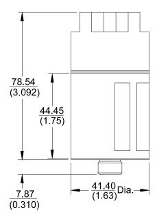
Figure 6: Terminal Block Connector 9200 Option -05 or 74712 Option -03
