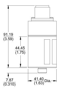
Figure 4: Top Mounted Connector Arial 9200 Option -01 or 74712 Option-02
