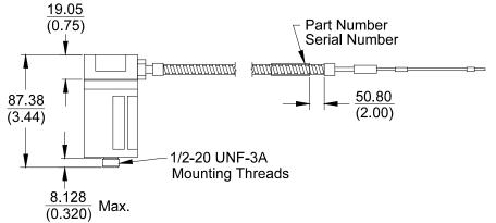
Figure 8: 9200 Connector Options -07 thru -50 All dimensions are in millimeters (inches)
