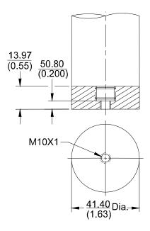
Figure 14: 9200 and 74712 Mounting Base Option -10 or -11 Option -10 Circular M10x1 or Option-11 Isolated Circular M10X1
