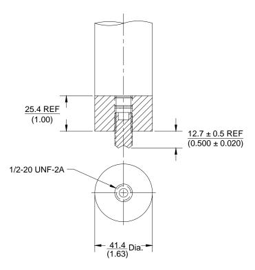
Figure 15: 9200 Mounting Base Option -12 Isolated Circular ½-20 UNF-2A
