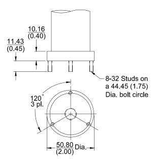
Figure 12: 9200 and 74712 Mounting Base Option -04 3 each 8-32 studs
