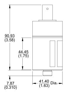
Figure 7: BNC Connector 9200 Option -06 or 74712 Option -01
