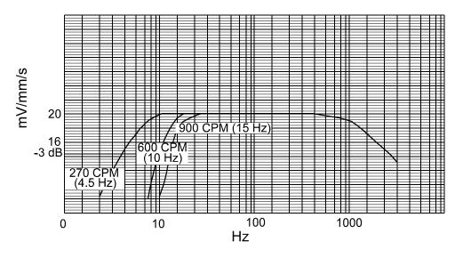
Figure 2: Theoretical Velocity Seismoprobe Frequency Response
